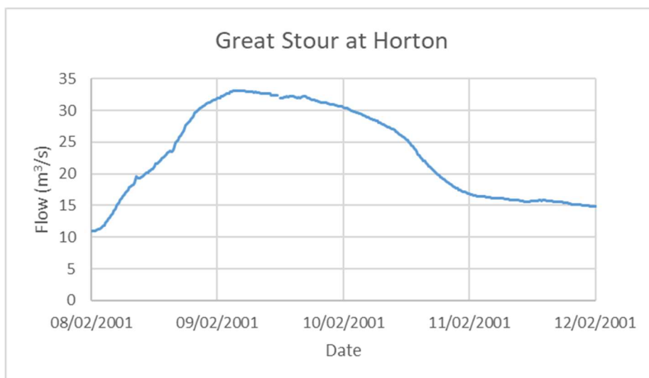
Figure 2-11: Horton plots of flood peak and flow data and interpretation (Feb 2001)
